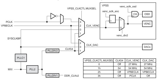
Figure 4-2. VPBE/DAC Clocking
